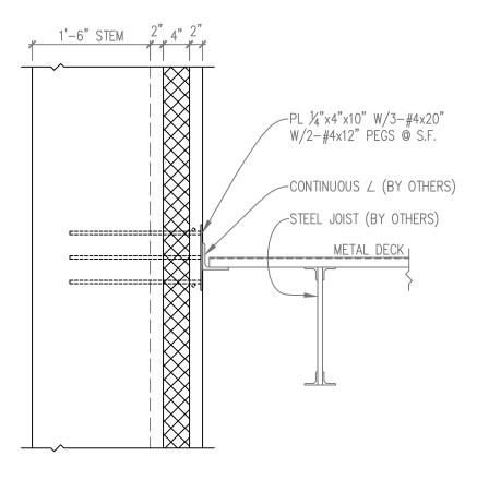
DT WALL PANEL TO STEEL DECK - NON LOAD BEARING
