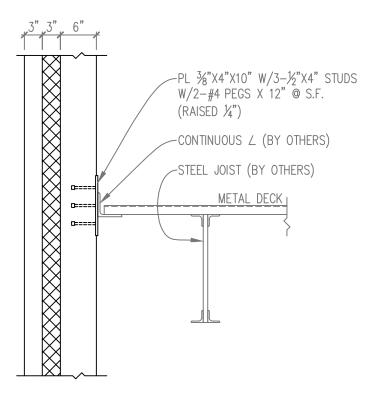
\ FLAT PANEL TO JOIST - NON LOAD BEARING
