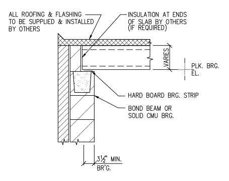
HOLLOWCORE PLANK BEARING ON MASONRY
