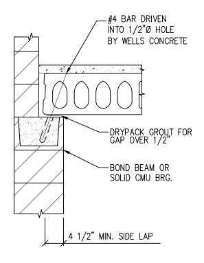
HOLLOWCORE FLOOR PLANK AT EXTERIOR WALL NON-LOAD BEARING
