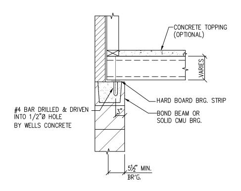
HOLLOWCORE PLANK BEARING ON MASONRY
