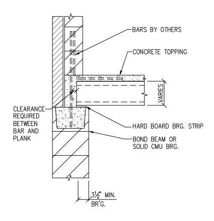
HOLLOWCORE PLANK BEARING ON MASONRY
