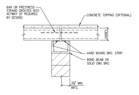
HOLLOWCORE FLOOR PLANK BEARING ON INTERIOR MASONRY WALL
