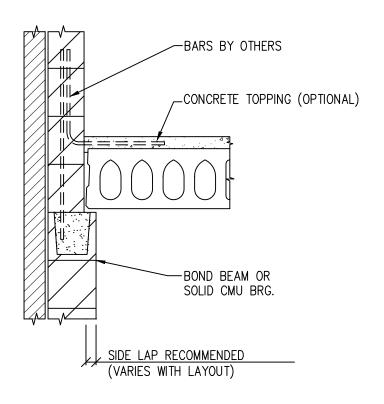
HOLLOWCORE FLOOR PLANK AT EXTERIOR WALL NON-LOAD BEARING
