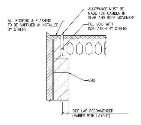
HOLLOWCORE ROOF PLANK AT EXTERIOR WALL NON-LOAD BEARING
