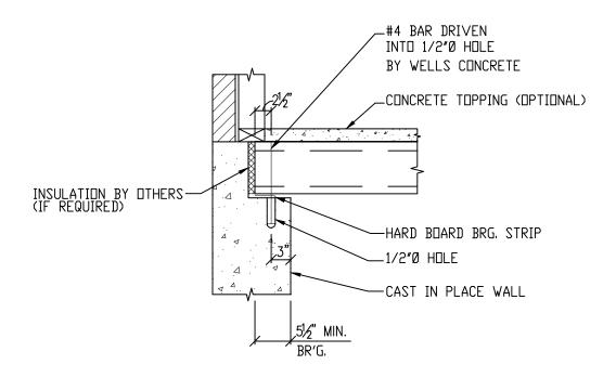
HOLLOWCORE FLOOR PLANK BEARING ON EXTERIOR C.I.P. WALL
