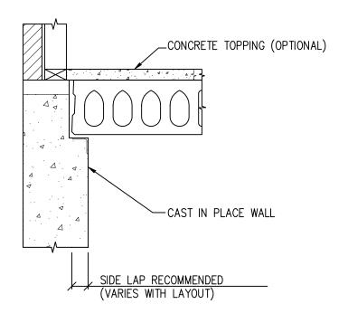
HOLLOWCORE FLOOR PLANK AT EXTERIOR C.I.P. WALL NON-BEARING
